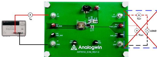
Figure 4. Measuring No-load Input Current
